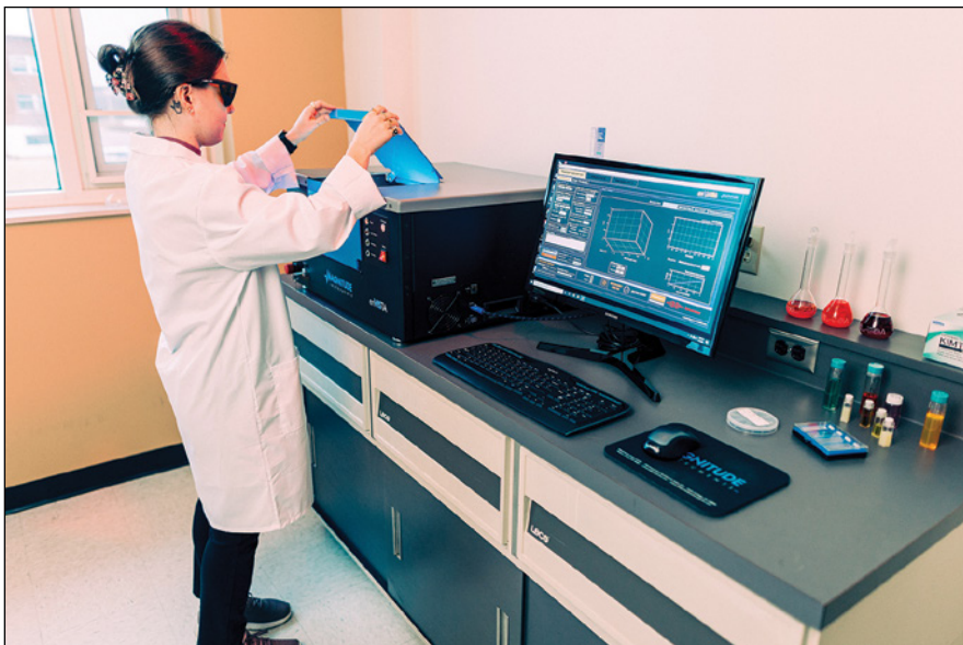
Fully integrated benchtop nanosecond transient absorption spectrometers are designed for advanced time-resolved spectroscopy applications. (Credit: Magnitude Instruments)
