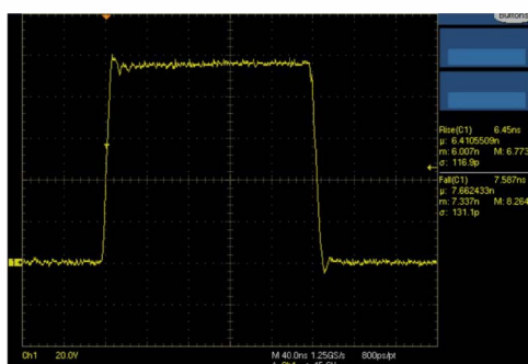
Fig 1 Output pulse shape 3.6kV 6PF capacitive load
