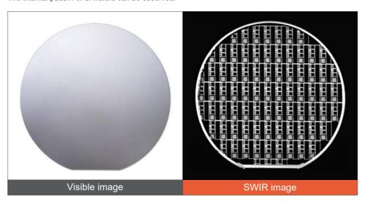
Sample: Si wafer Wavelength: 1100 nm Illumination: Transmission
