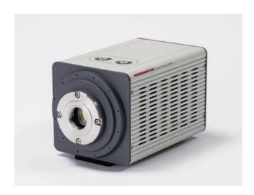
The C12741-11 is a near-infrared camera which employs a 640 pixels  $\times$  512 pixels InGaAs sensor. -70 °C peltier cooling significantly reduces dark current which leads to improved image quality and allows imaging with long exposure time.
