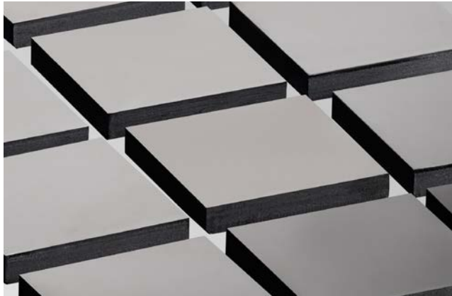
Precise dicing of a silicon wafer.
