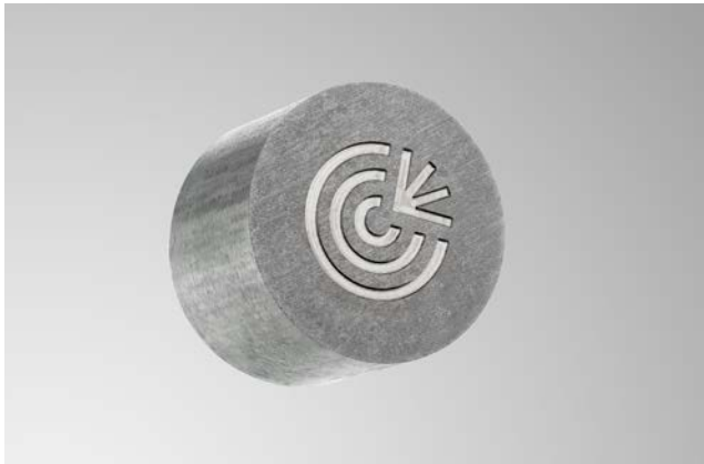
Selective ablation of tungsten carbide.
