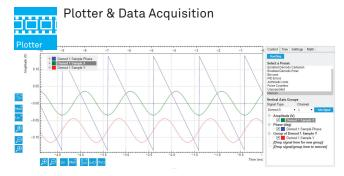
The Plotter and Data Acquisition module display multiple measurement data in the time domain. The Plotter displays the data continuously and the Data Acquisition module captures and displays individual shots based on numerous internal and external trigger conditions.
