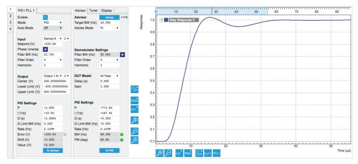
Each of the 4 PID/PLL controllers has a dedicated tab with the main controller settings in the left section, the DUT model settings and auto-tune further to the right and a large diagram to see the modelled transfer function and step-response.
