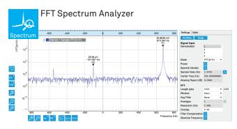
The Spectrum Analyzer takes any of the demodulators' outputs or frequency as an input and applies a Fast Fourier Transformation. The main features are:
