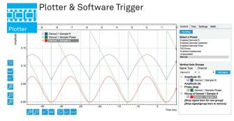
The Plotter and Software Trigger display multiple measurement data and model parameters in the time domain. The Plotter displays the data continuously and the Software Trigger captures and displays individual shots based on numerous different internal and external trigger conditions.
