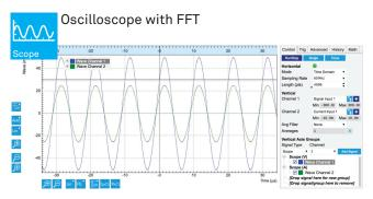
Time and frequency domain analysis of signal inputs and trigger signals with the following key features:
