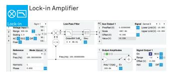
Every demodulator has a graphical representation in the form of a block-diagram for intuitive instrument understanding. In addition, the overview tab allows the control of all demodulators, signal inputs and signal outputs from a single panel.
