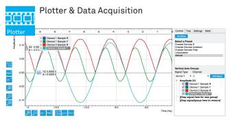
The Plotter and Data Acquisition module display multiple measurement data in the time domain. The Plotter displays the data continuously and the Data Acquisition module captures individual shots based on numerous internal and external trigger conditions.
