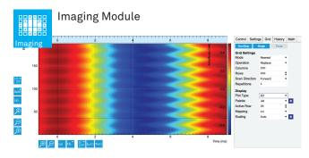
The imaging module converts any of the measurement signals into images and supports
