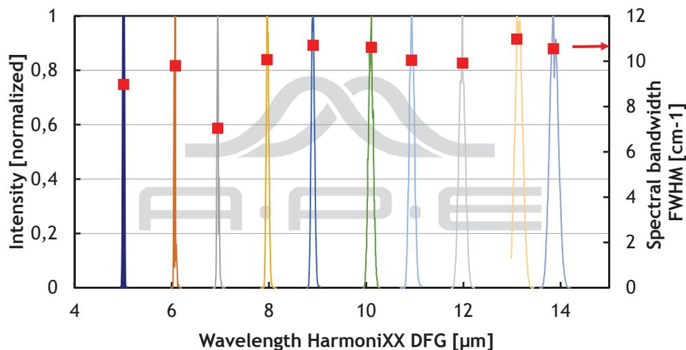
The narrow line width of the pump is preserved in the DFG process. With a spectral bandwidth of around  $10\text{ cm}^{-1}$  the pulses are ideal for applications that require a high resolution, e.g. spectroscopy.
