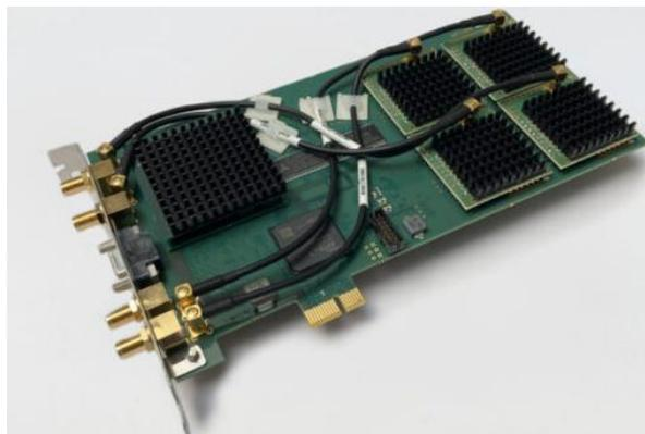
You should have a Becker&Hickl SPC-QC-104 inserted in a PCIe slot of Windows 64-Bit computer running at least Windows 10 or later.
